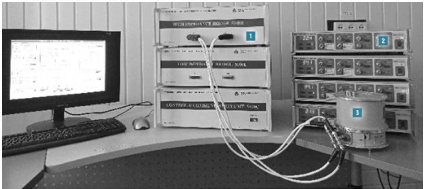
Fig. 3. Providers measurement system for electrical capacity measurement (1 – comparator 5100; 2 – measurement standard; 3 – P 597 measure)
