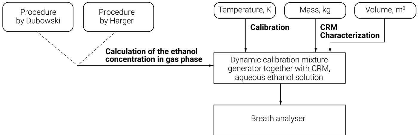
Fig. 3. Simplified metrological traceability chain for the analysers calibrated with type A generators
