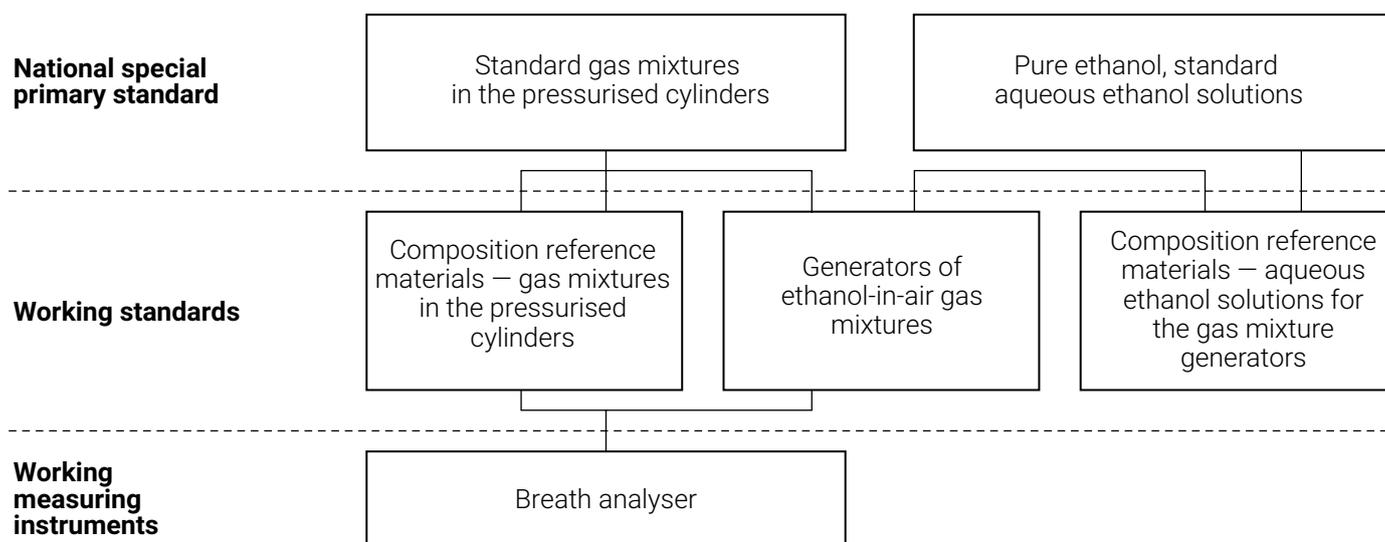
Fig. 8. Traceability chain based on the «verification chart» for breath analysers adopted in Russia [28]
