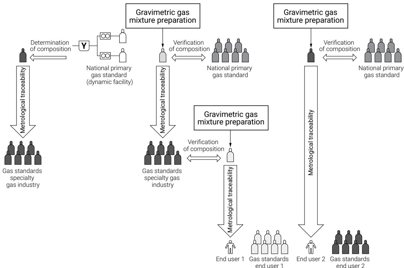
Fig. 1. Scheme of metrological traceability dissemination through calibration gas mixtures according to ISO 14167 [7]
