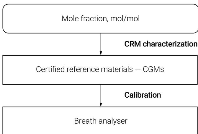
Fig. 2. Simplified traceability chain for the analysers calibrated with the certified reference materials – CGMs
