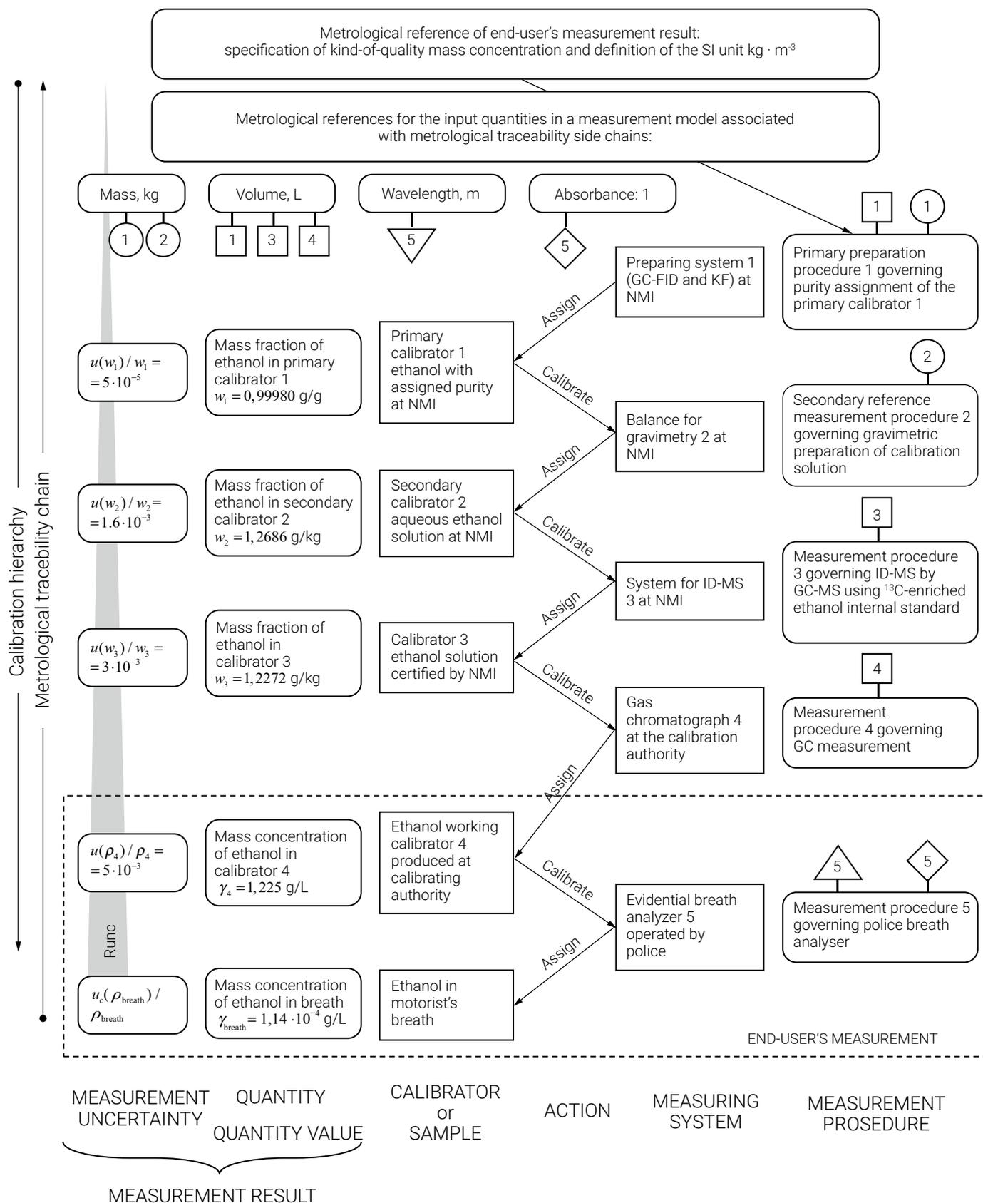
Fig. 6. Metrological traceability chain for the breath analysers according to [9]
