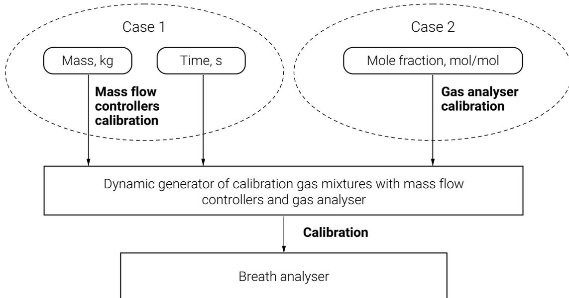
Fig. 5. Simplified metrological traceability chains for the analysers calibrated with type B generators
