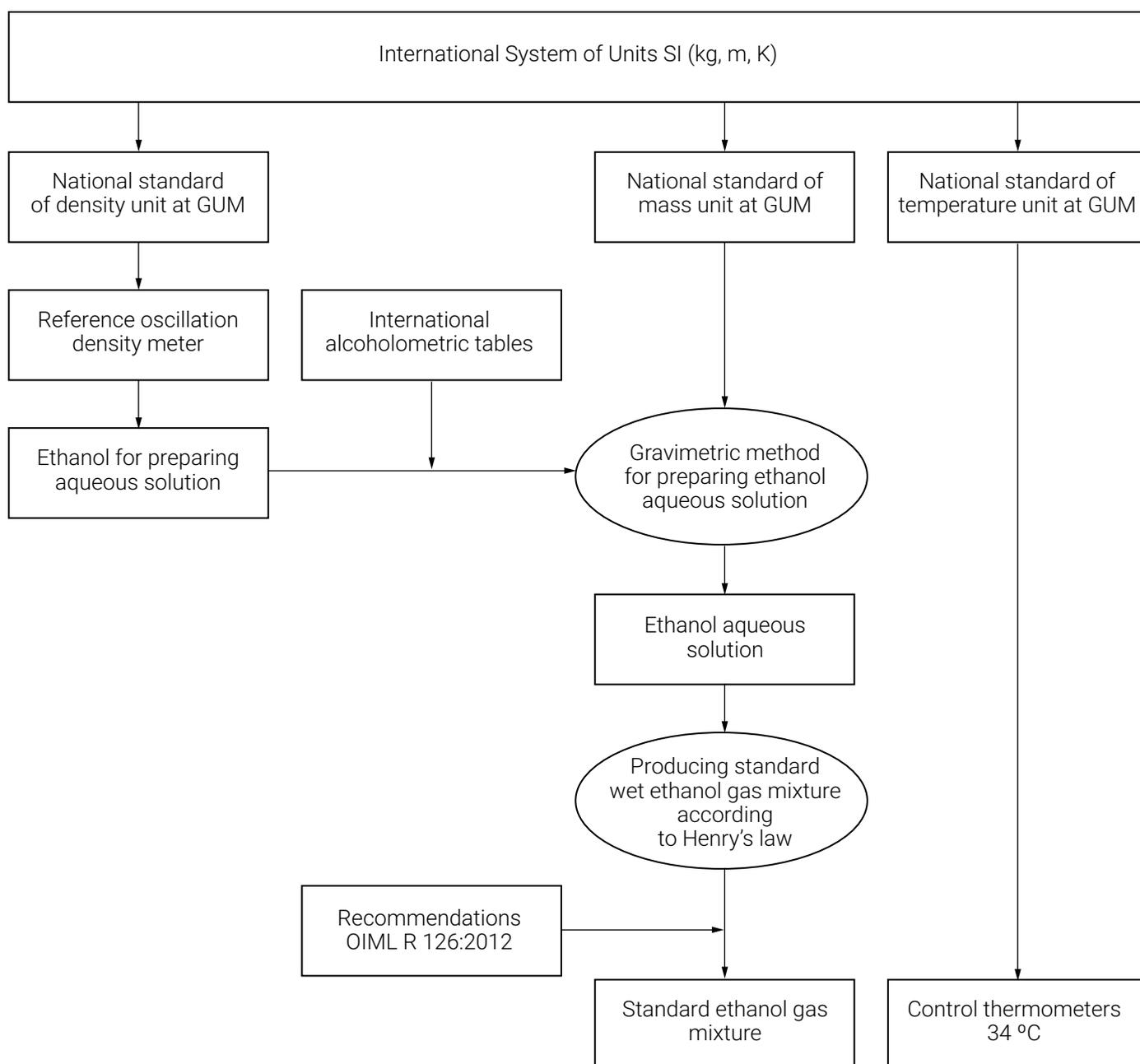
Fig. 7. The traceability chain, based on dynamic generators and standard ethanol solutions, adopted in Poland [26]
