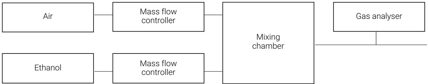
Fig. 4. Simplified scheme of the type B generator
